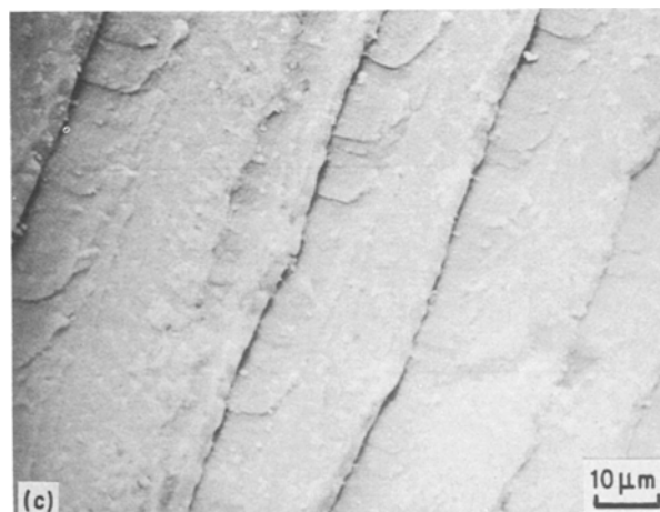
Figure 4 Fractured surfaces of (a) copper doped \gamma -Al 2 O 3 , (b) slip steps in the boehmite phase, (c) colony structure in \delta -Al 2 O 3 .
